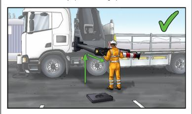
Stabilisers with a manually operated swing-up function cannot be retracted at a 90° horizontal position, so there is no risk of crushing when the stabiliser beam is retracted.
