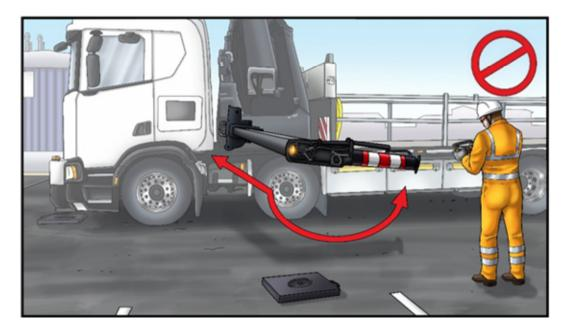
This will be reviewed as manufacturers develop products which prevent the possibility of operators being crushed by a stabiliser leg while operating the fixed controls.
